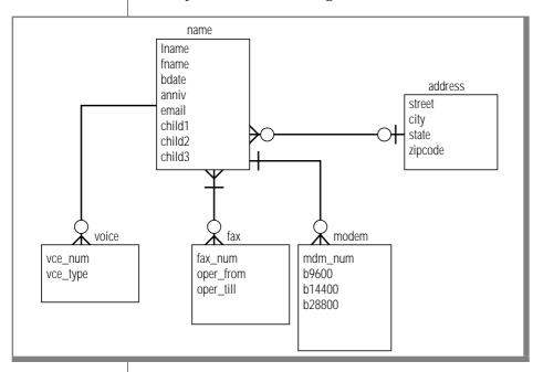
Figure 2-15 Preliminary Entity-Relationship Diagram of the Telephone-Directory Example
